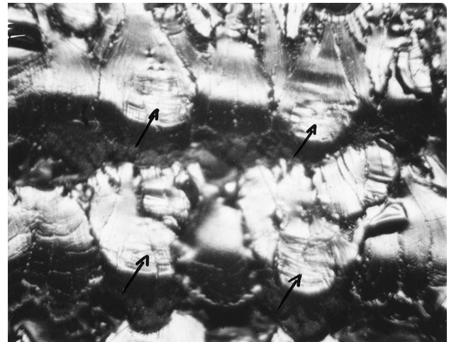
Figure 12 Photograph of peeled surface of impulse-welded sample. Note points of delamination, magnification \times 15
