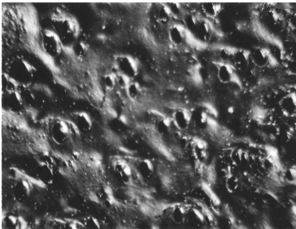
Figure 11 Photograph of peeled surface of HF-welded sample giving rise to peeling forces of 4000 N/m at 70°C. Note pitted appearance, magnification \times 15 .
