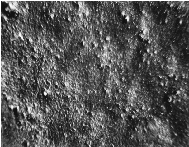
Figure 10 Photograph of peeled surface of HF-welded sample giving rise to peeling forces of 2300–2700 N/m at 70°C. Note smooth appearance, magnification \times 15 .
